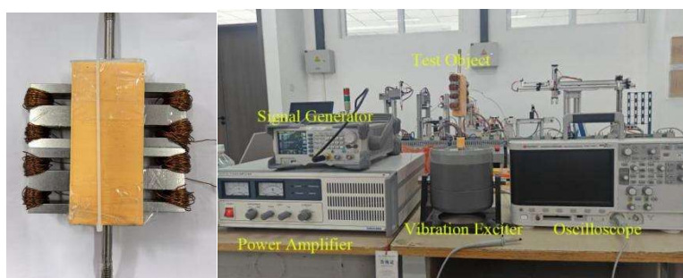
Figure 5. Prototype of the vibration power generation device (left) and experimental setup (right)
