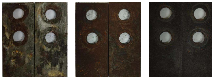
(a) Inbound pipeline (b) Sewage pipeline (c) Outbound pipeline
