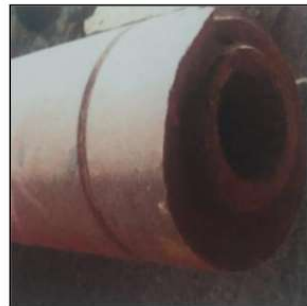
(b) Drill pipe failure[25]
