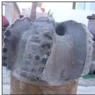
(a) Drill tooth damage[25]
